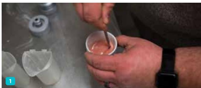
**Fig 1.** Mixing Pala acrylics for injection processing.
