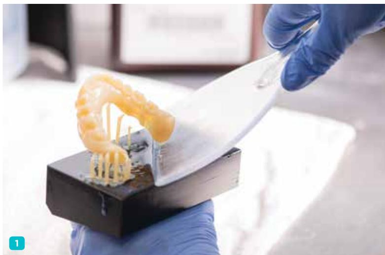
**Fig 1.** Removing a print from the build table.
