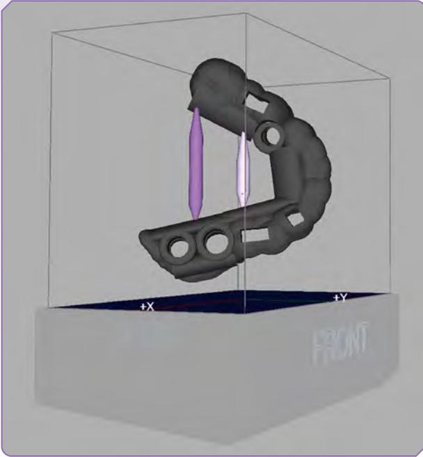
Adding stabilization bars: min. 2 up to 3 are required
