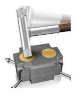
⚠ REMOVE STONE FROM THE FLASK WITH A PLASTIC HAMMER. DO NOT HIT THE FLASK WITH HAMMER!!
