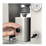
After the mold is full, acrylic will escape through the ventilation channel, which is then closed by turning the vent knob clockwise.
