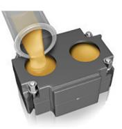
Apply Aislar separating agent and fill the remainder of the flask with stone. Remove excess stone from the flask so it will fit between the centering disks of the Palajet<sup>®</sup>.
