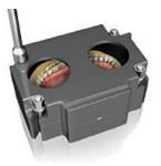
Pour stone through openings e and fill the entire flask until the stone reaches the occlusal surface of the teeth.
