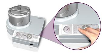
**b** After 30 minute polymerization time, take flask out of the Palamat elite and let it cool down to room temperature (30-60 minutes).
