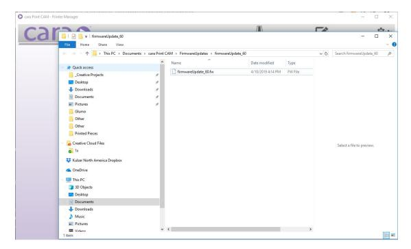
With the firmware update on your USB-stick, walk over to your printer and insert the stick into the front USB slot of cara Print 4.0. Once inserted, the file transfer menu should automatically popup. Select the firmwareUpdate\_60 file and then simply follow the instructions on the screen.
