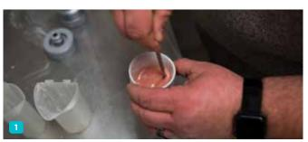
Fig 1. Mixing Pala acrylics for injection processing.
