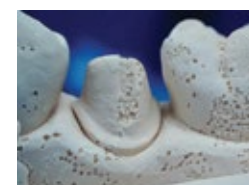
Porosity in stone due to immediate pour up
