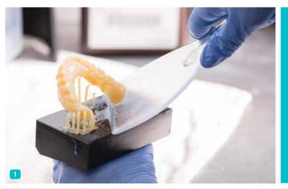
Fig 1. Removing a print from the build table. Fig 2. Prepping the printed denture base for finalization. Fig 3. Nesting with cara Print CAM. Fig 4. Printed denture finishing with gingiva characterization using Pala cre-active.
